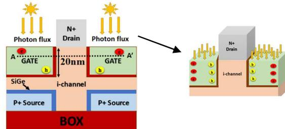
Fig. 1 Schematic illustration of optically gated Dual MOSCAP VTFET for photosensing application.
