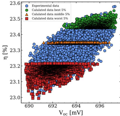
FIG. 1. 32'000 experimental IV parameters of a typical new PERC factory in China (blue symbols), with the machine learning (ML) results of the 10% cells with the lowest, medium and best efficiency  $\eta$  are shown in the traffic light colours.
