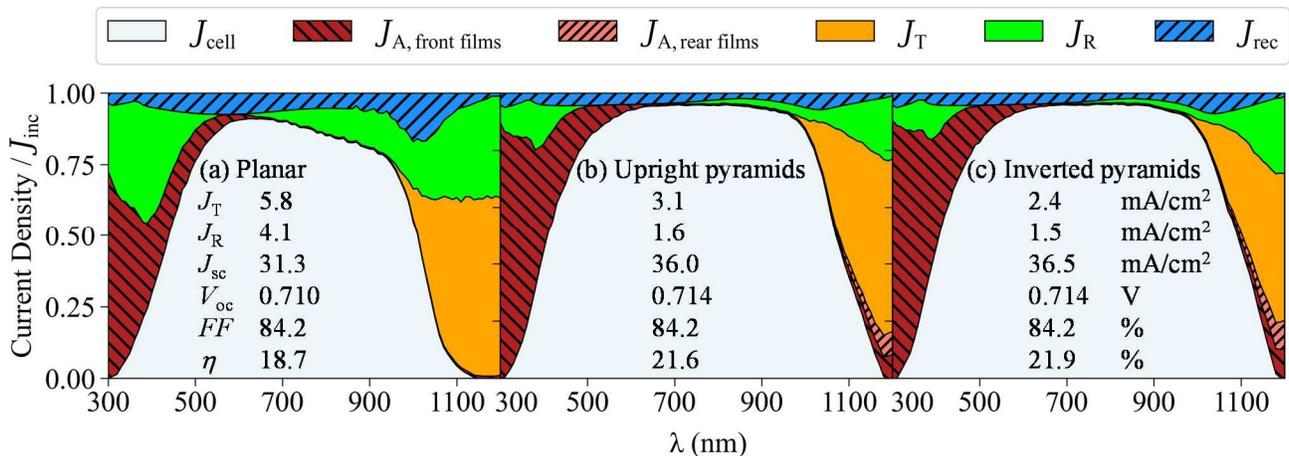
Fig. 3. Sources of current loss at  $P_{\max}$  for normal-incidence front illumination with front and rear surface textures as labelled.
