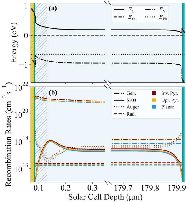
Fig. 2. (a) Electronic band structure and (b) generation and recombination rates for the bifacial SHJ under front illumination at  $P_{\max}$  for varied textures.
