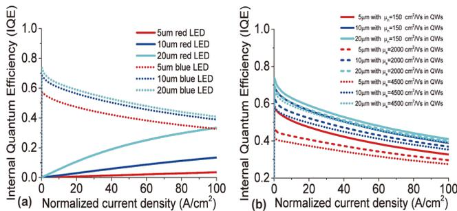
Fig. 2. (a) The IQEs of three kinds of chip size between red LED and blue  $\mu$ LED. (b) The influence of different carrier mobility in blue LED QWs with consideration on random alloy fluctuation.
