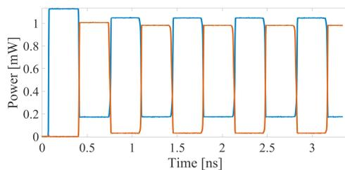
Fig.3 Mode switching in Regime I ( $L_I=100 \mu\text{m}$ ,  $L_2=5$  cm)
