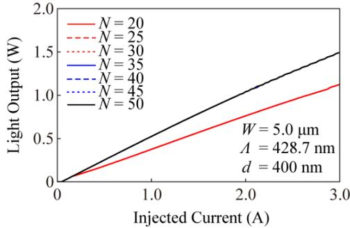
Fig.2 Injected current versus light output curves when  $W=5.0 \mu\text{m}$ ,  $S=426 \text{ nm}$ ,  $\Lambda=428.7 \text{ nm}$ , and  $d=400 \text{ nm}$ . The parameter is the number of the grating periods  $N$ .
