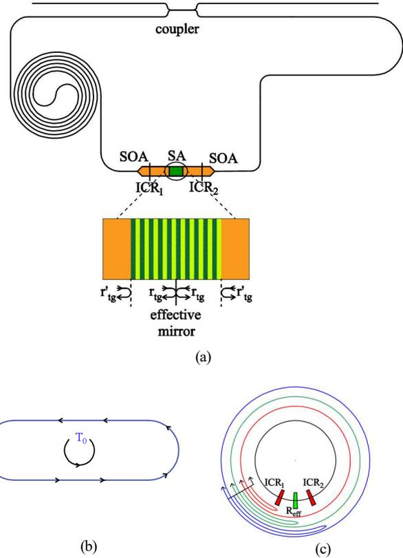
Fig. 1. (a) Schematic of proposed structure and corresponding paths for time delays used for derivation of DDE model in (b) WOICRS and (c) proposed structure.
