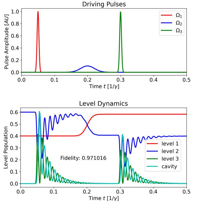
Fig. 2. Top: Pulse sequence.  $\Omega_1$  and  $\Omega_3$  drive the optical transition,  $\Omega_2$  flips the QuBit. Bottom: Population dynamics for optimized pulses for mixed QuBit starting condition.
