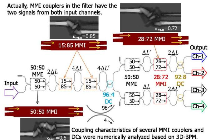
Fig. 1. Proposed MDI-type wavelength filters for Coarse WDM applications.
