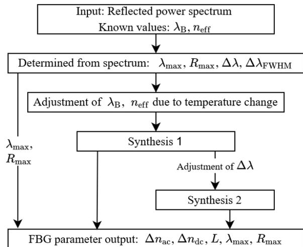
Fig. 1. Flow chart of the implemented FBG synthesis. The FBG parameters needed for the Digital Shadow are the output values.
