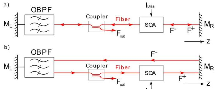
Fig. 1. a. Bidirectional SOA Fiber Laser Cavity
