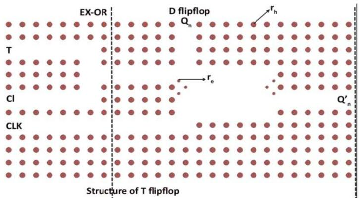
Fig.1. Schematic structure of all optical T-flip flop
