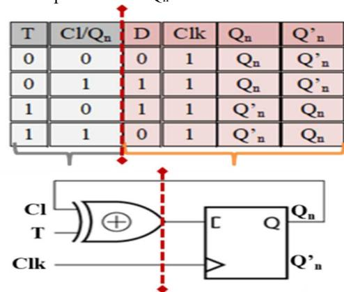
Fig. 2 Truth table with logic diagram for T-flip flop
