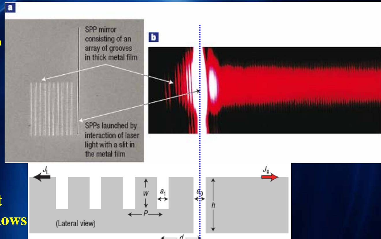
Careful choice of the distance between the slit and the groove array allows the reflected SPPs to constructively interfere with the SPPs traveling in the opposite direction — the direction the authors wish them to travel.
