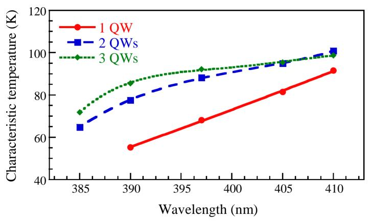
The DQW structure has the largest  $T_0$  when the wavelength is larger than 405 nm, while the TQW structure possesses the largest  $T_0$  when the wavelength is smaller than 405 nm.
