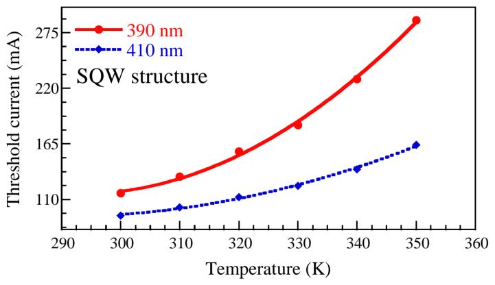
It can be found clearly that the threshold currents at 410 nm are much more stable with temperature and smaller than those at 390 nm.
