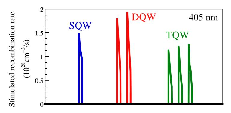
It indicates that the DQW structure has the best stimulated recombination distribution which may be caused by effective carrier and optical confinements in the active region.
