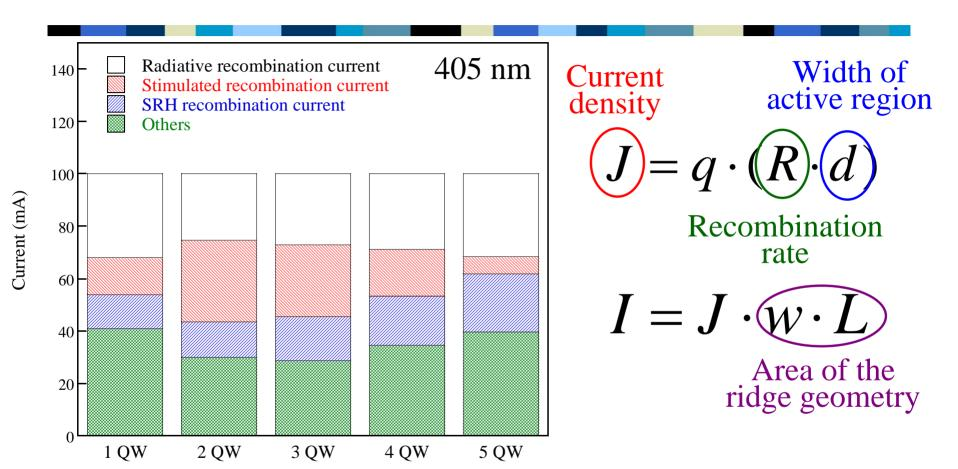
The stimulated recombination current is about 31.13% of the total current for the DQW laser structure and 6.57% of the total current for the five-quantum-well laser structure.
