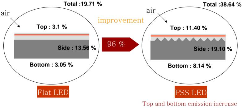
Top emission is similar to bottom emission and most of total emission is emitted to the side. Top and bottom emission increase relatively rather than side emission. And the top emission is larger than bottom emission.
