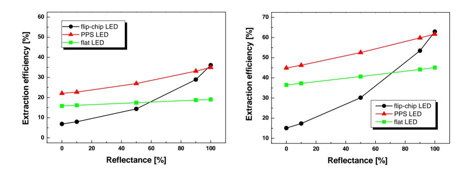
It should be noted that the extraction efficiency at flip-chip LEDs is more sensitive to the reflector of bottom face than that of flat and PSS LEDs.
