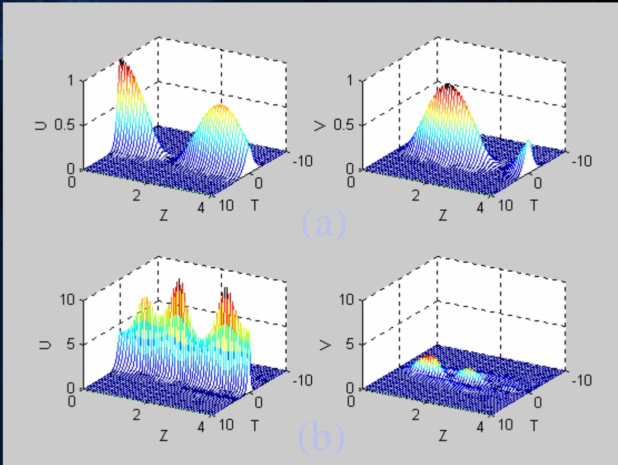
Nonlinear pulse propagation with  $R=1$ ,  $R' = R'' = 0$
