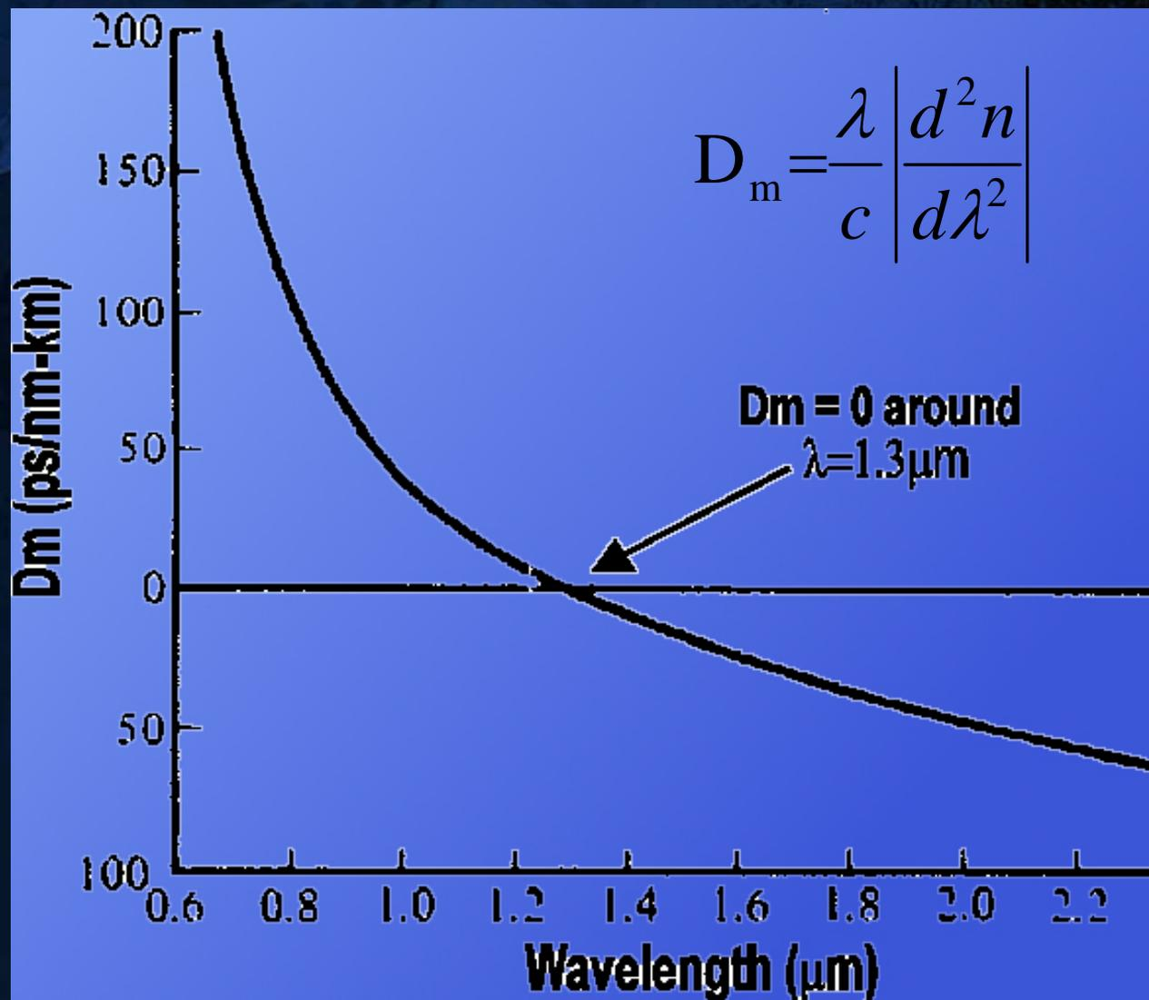
**The material dispersion parameter for silica as a function of wavelength (Payne & Gambling 1975)**
