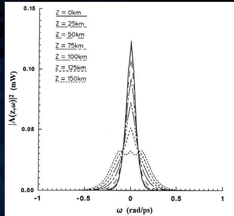
Frequency domain solution for the propagation of soliton in an optical fibre with only nonlinear effect
