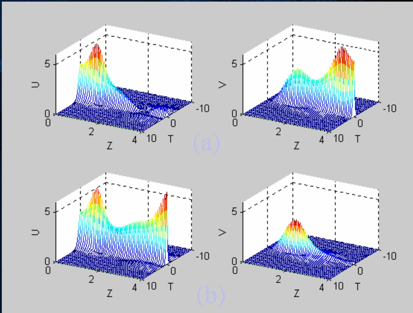
Nonlinear pulse propagation with  $R=1$ ,  $R' = R'' = 0$  and an initial peak pulse amplitude of (a) 1.89 and (b) 1.90
