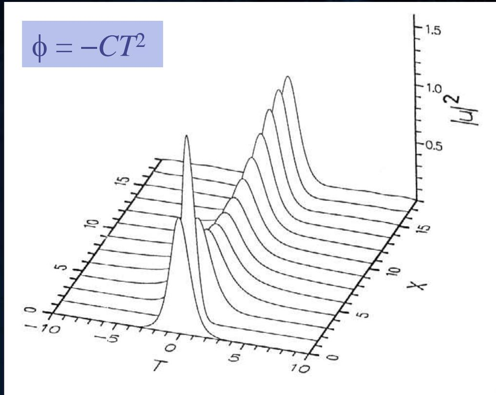
**Propagation of a fundamental solitons in a lossless fibre with an initial frequency chirp of  $C=0.25$**
