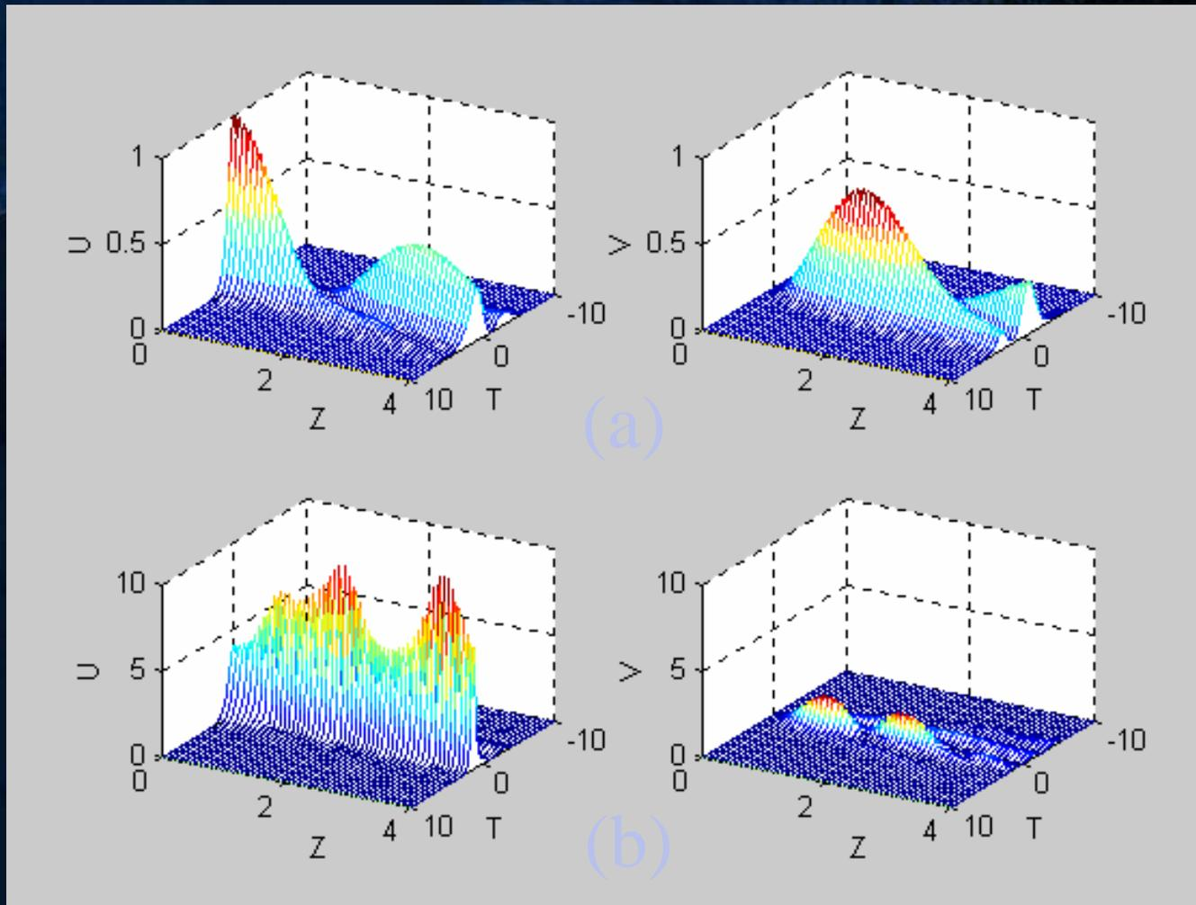
Nonlinear pulse propagation with  $R=1$ ,  $R' = -0.5$ ,  $R''=0$  and an initial peak pulse amplitude of (a) 1 and (b) 2
