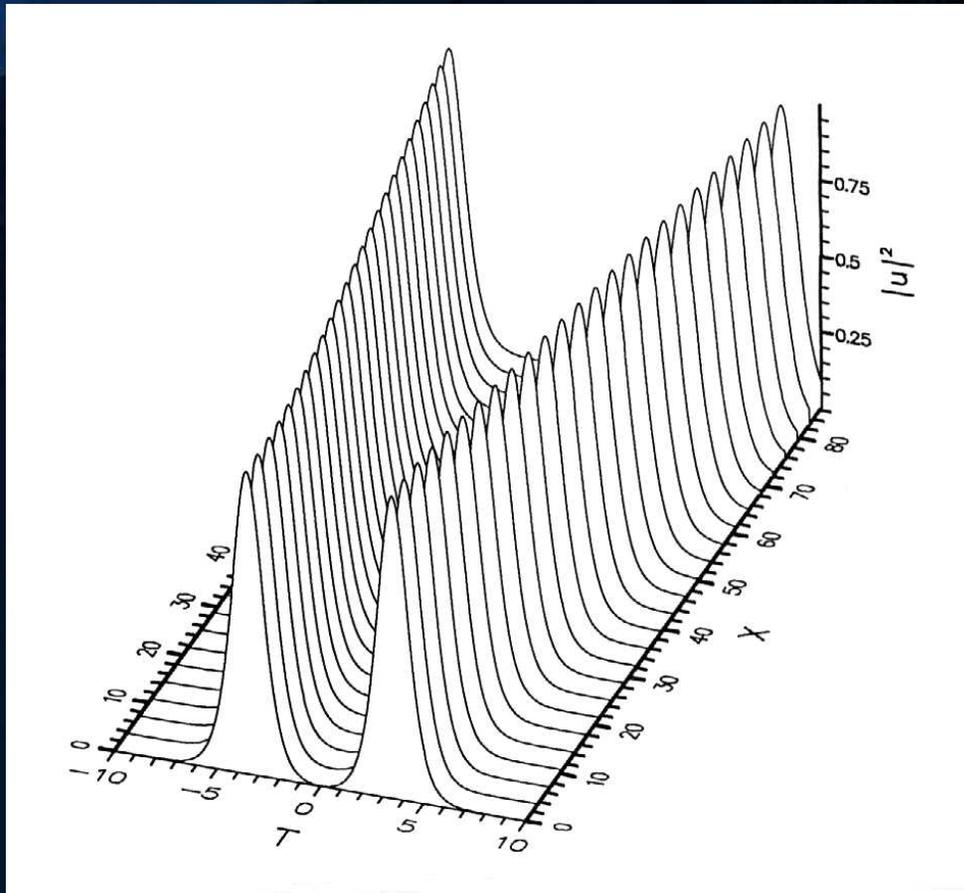
**Propagation of two fundamental solitons in a lossless fibre
