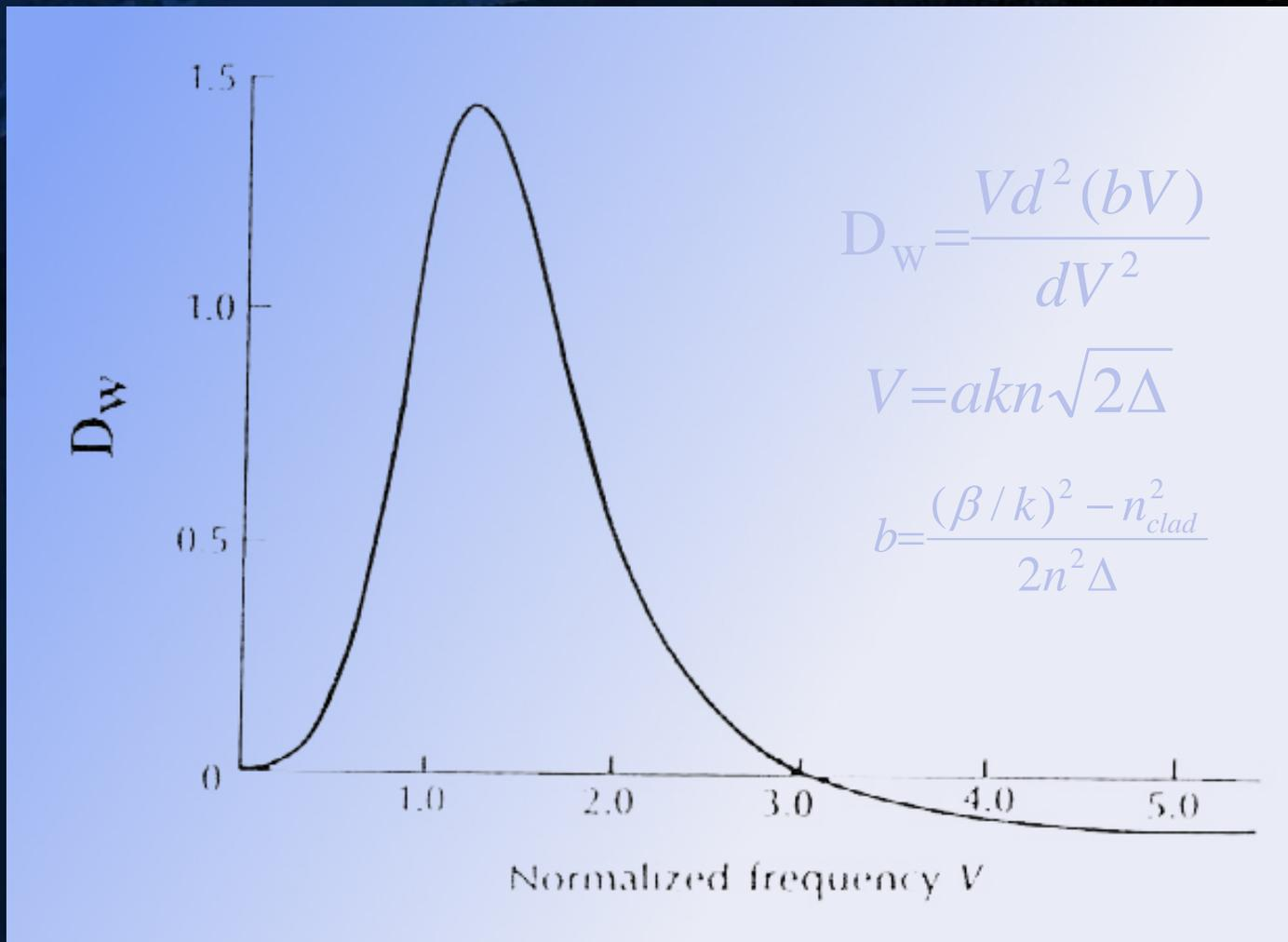
The waveguide dispersion coefficient versus normalized frequency (Gambling *et al.* 1981)
