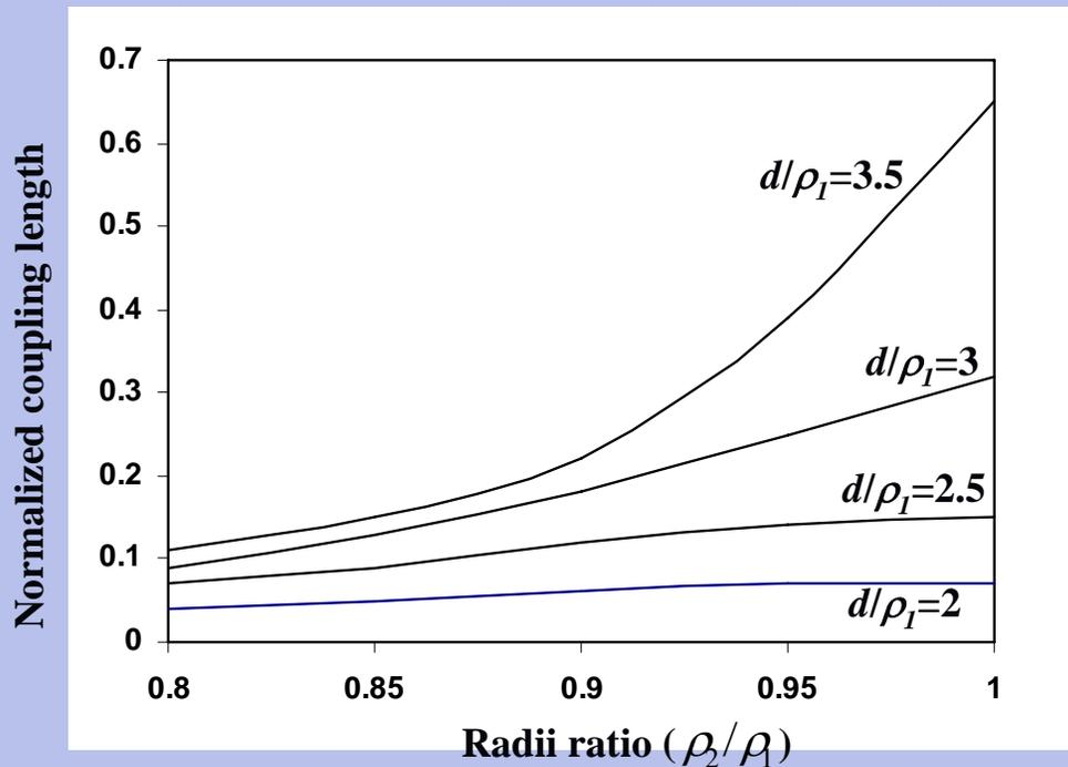
For a certain core separation, the normalized coupling length decreases as the difference of two cores increases
