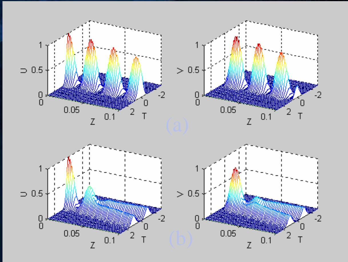
Linear pulse propagation with  $R=100$ ,  $R''=0$ ,
