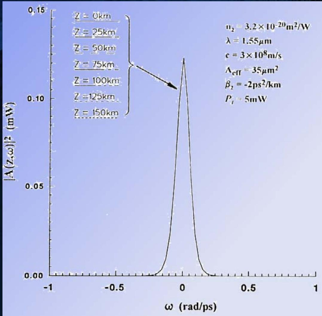
Propagation of a fundamental soliton pulse in a purely dispersive optical fibre
