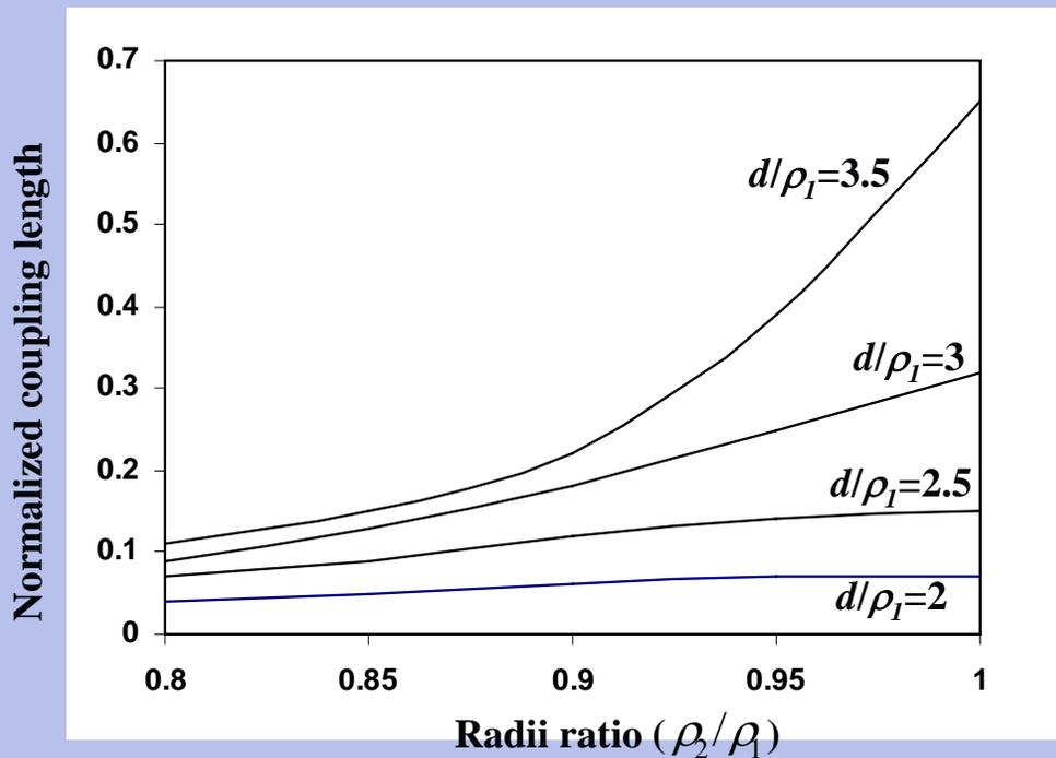
Normalized coupling length as a function of radii ratio  $\rho_2/\rho_1$  for different core separations
