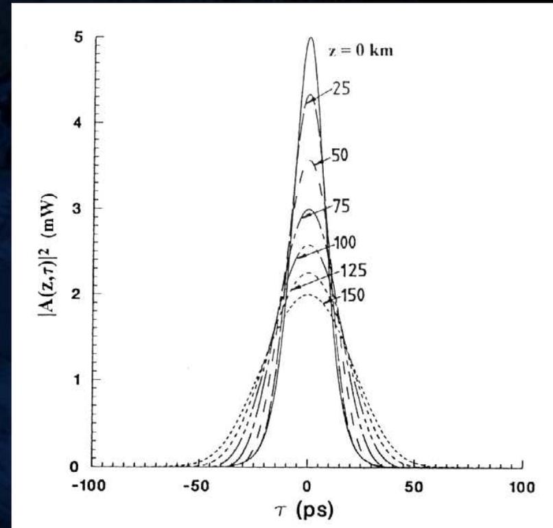
Propagation of a fundamental soliton pulse in a purely dispersive optical fibre
