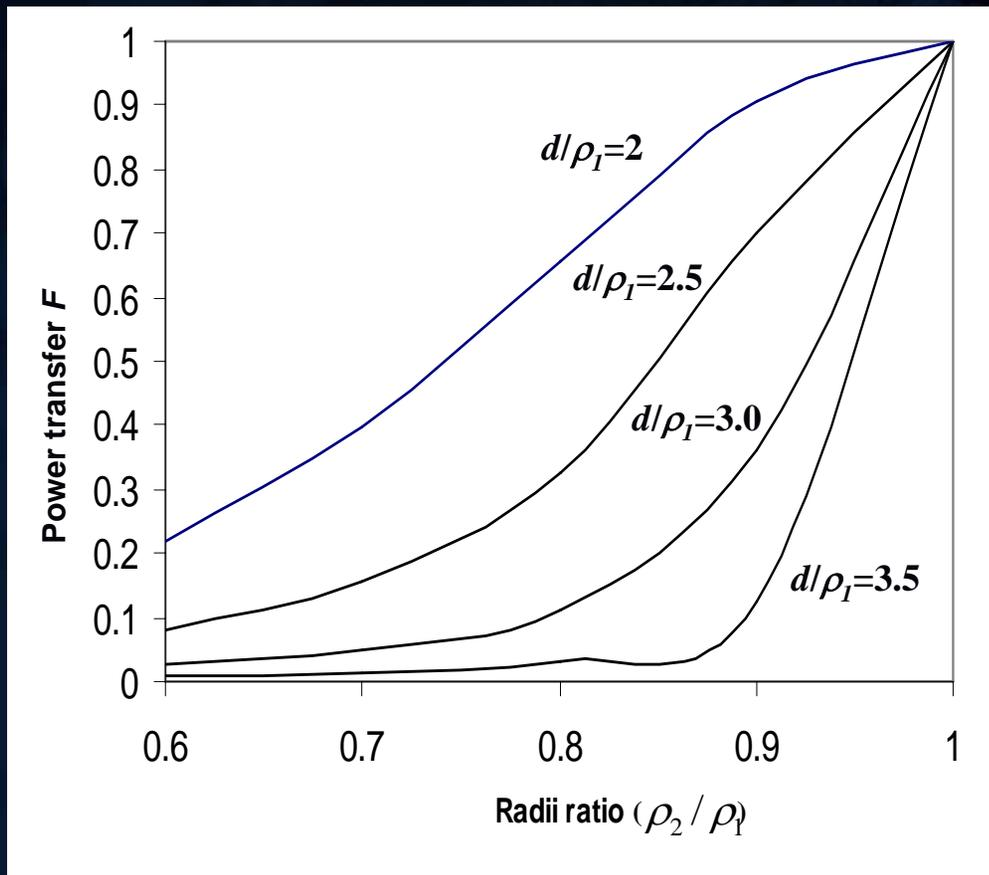
❖ For a given radii ratio, the power transfer decreases with the increase of the core separation
