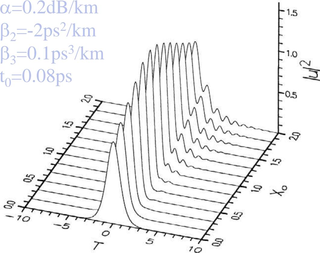
Propagation of a fundamental solitons in a dispersion-shifted fibre with an initial requency chirp of  $C=0.25$
