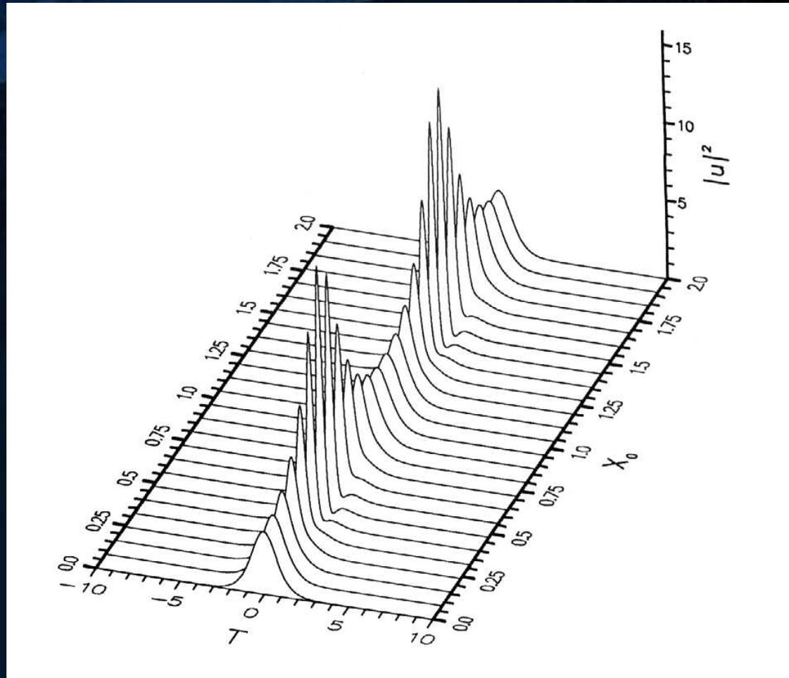
**Propagation of two fundamental solitons in a lossless fibre
