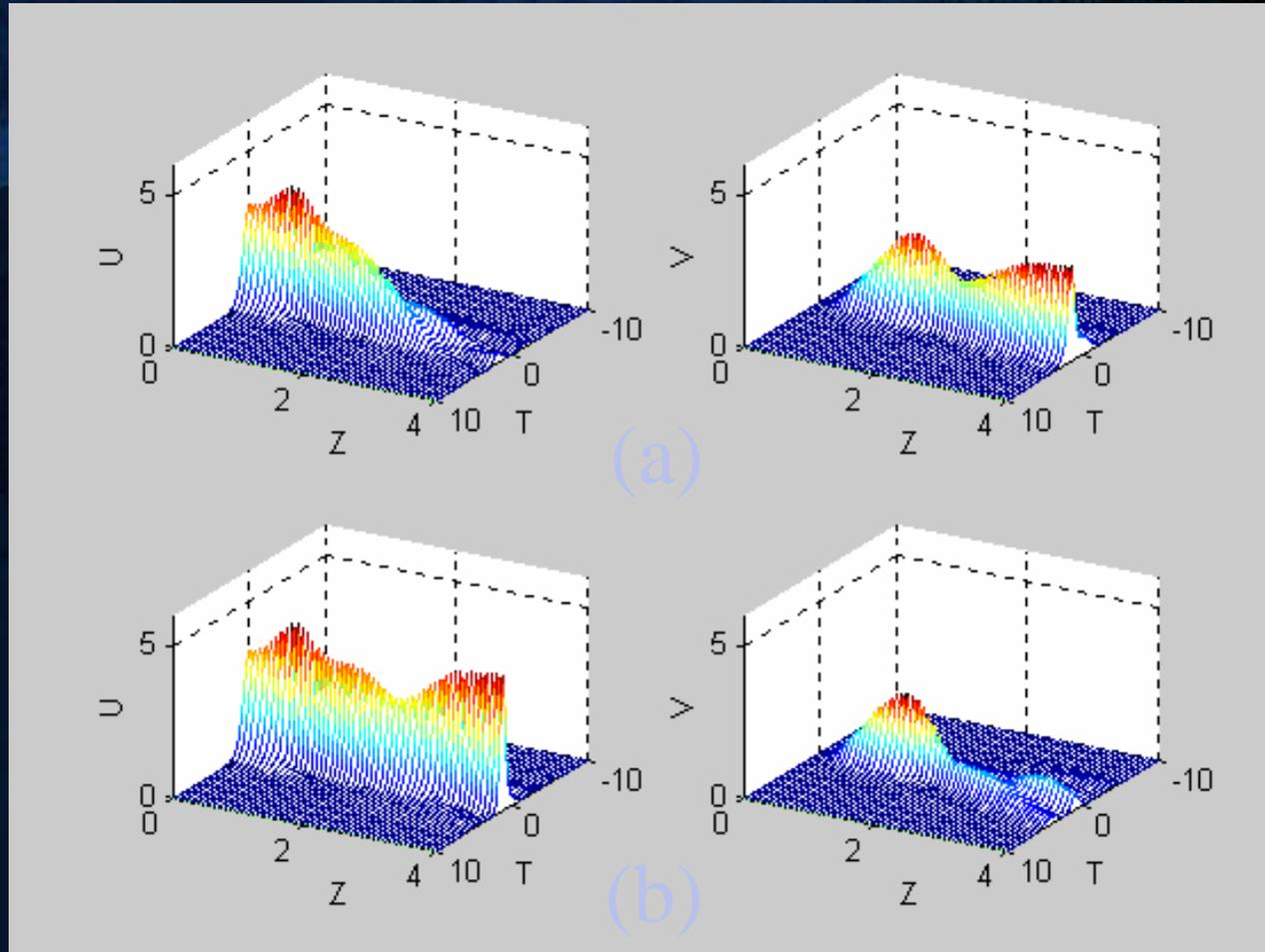
Nonlinear pulse propagation with  $R=1$ ,  $R' = -0.5$ ,  $R'' = 0$  and an initial peak pulse amplitude of (a) 1.80 and (b) 1.84
