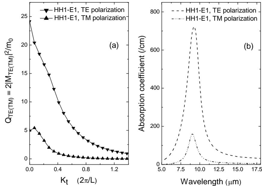
Calculated (a) squared optical transition matrix elements vs plane wave vector  $k_t$  and (b) absorption coefficients vs. optical wavelength of E1-HH1 transition for TE and TM polarizations
