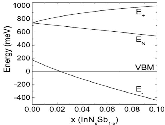
**Calculated band dispersion with the N content using BAC model**
