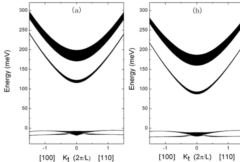
**(a)  $\text{InSb}_{0.99}\text{N}_{0.01}/\text{InSb}$  MQW and (b)  $\text{InSb}_{0.985}\text{N}_{0.015}/\text{InSb}$  MQW**
