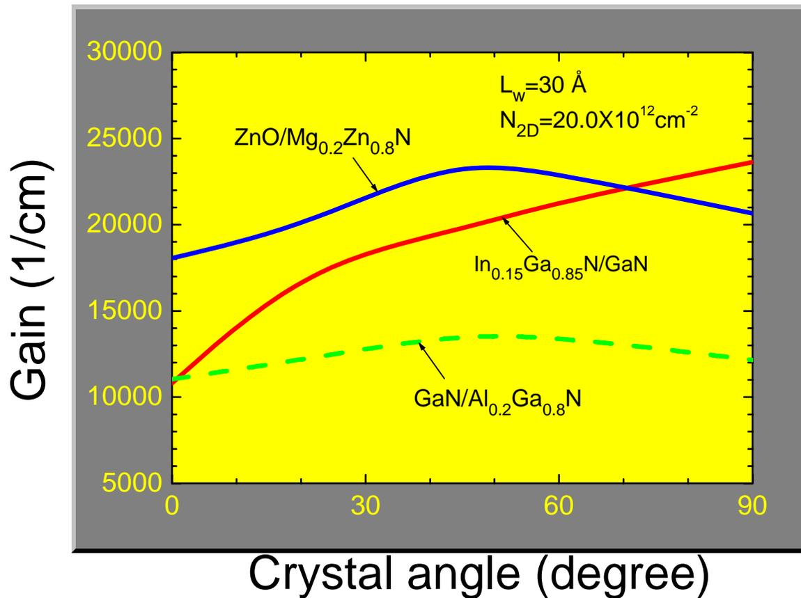
➤ In the case of small crystal angle, ZnO system has much larger optical gain than the GaN systems. This is because WZ ZnO/MgZnO QW structure has the larger matrix element and smaller effective mass than GaN-based QW structures near (0001) crystal orientation.
