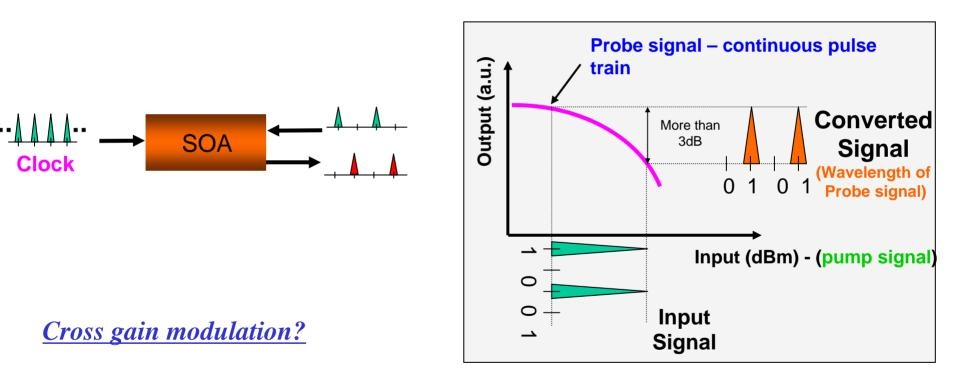
The carrier density changes in SOA a signal at one wavelength affect the gain of signal at another wavelength using carrier density change in SOA.
