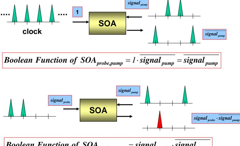
Boolean Function of  $SOA_{probe, pump} = signal_{probe} \cdot signal_{pump}$
