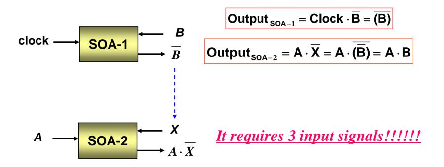
J. H. Kim et al., "All-Optical AND Gate Using Cross-Gain Modulation in Semiconductor Optical Amplifiers," Jpn. J. of Appl. Phys. 43, 608-610 (2004).
