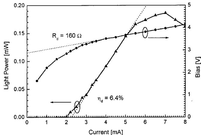
Fig. 2. Light–current ( $L - I$ ) and voltage–current ( $V - I$ ) characteristics measured ( $R_d$  is differential resistance and  $\eta_d$  is slope efficiency).
