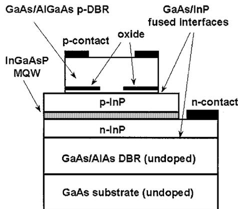
Fig. 1. Schematic view of our 1.55  $\mu\text{m}$  vertical-cavity laser.
