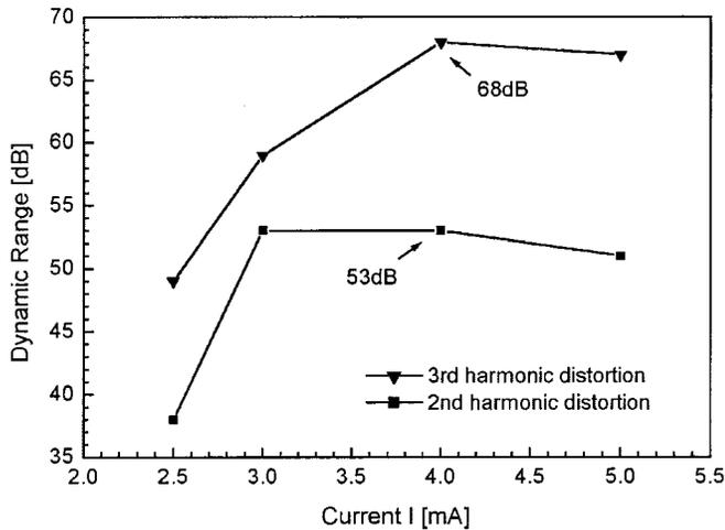
Fig. 5. Dynamic range (not SFDR) at 1-GHz modulation frequency for different input currents (as extracted from measurements like in Fig. 4).
